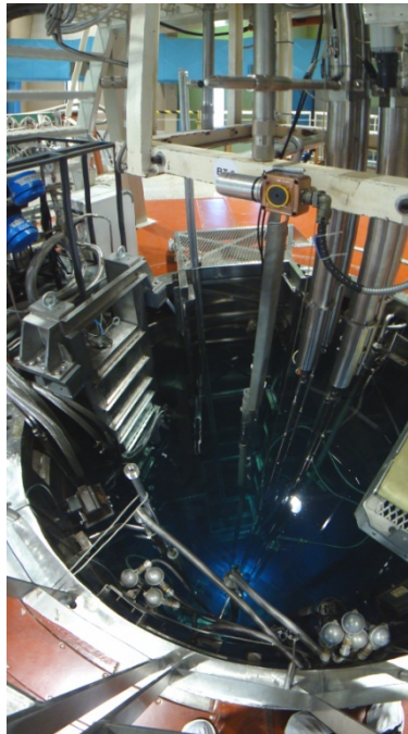
Fig. 19 – RA6 reactor irradiating the solution in the mini loop –B&W project
