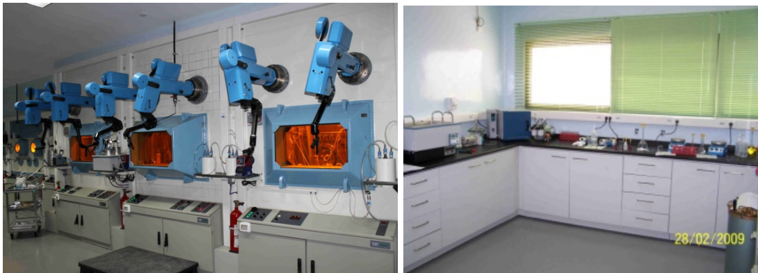
Fig. 11 – View of the hot cells front and one laboratory for measurements -RPF Egypt
