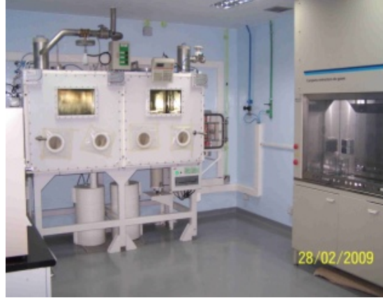
Fig. 11 – View of the decontamination & preparation cells and the hot cell in the laboratory -RPF Egypt
